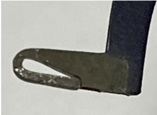
Over-compressed snap lock
