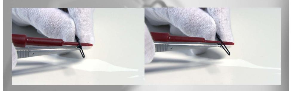
With the temple removed from the frame, carefully widen the temple opening by using either the red temple removal tool, or a pencil. Use tweezers to remove the disc. Installation of the new disc is accomplished using the same method.
