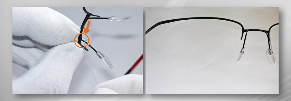
Cut nylor thread to required size and thread through.
