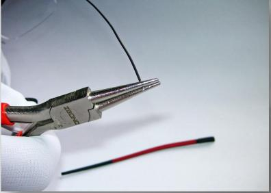
Squeeze metal inlay at the end with round pliers to secure temple end.
