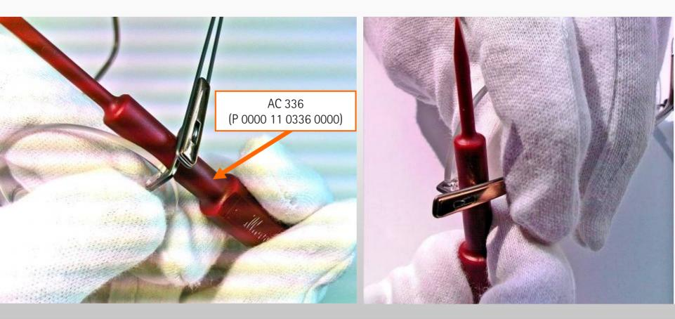
Use red disassembly tool. Place it as close as possible to the inside hinge.
