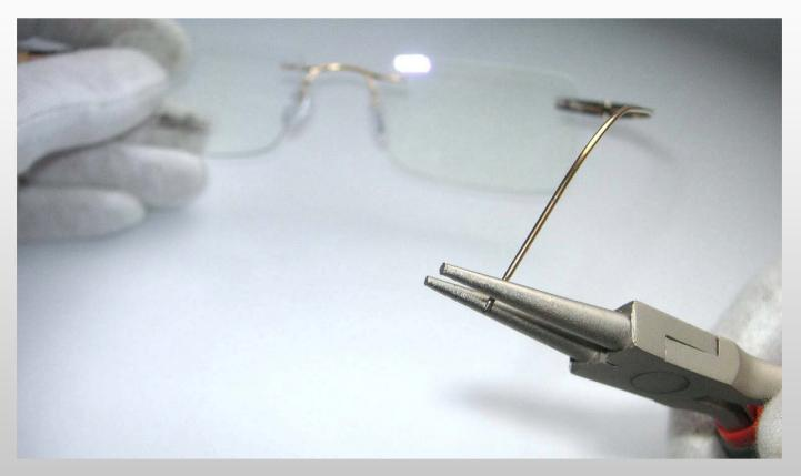
Squeeze metal inlay with round pliers at the very end. Attach temple end firmly to avoid slipping. Note: If necessary the temple end can be glued with Loctite 406
