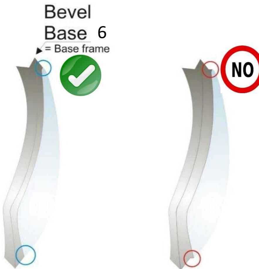
1. Neubau eyewear sun frames have a base curve 6. It would be advantageous when the bevel of the prescription lens has the same base curve! (base 6)
