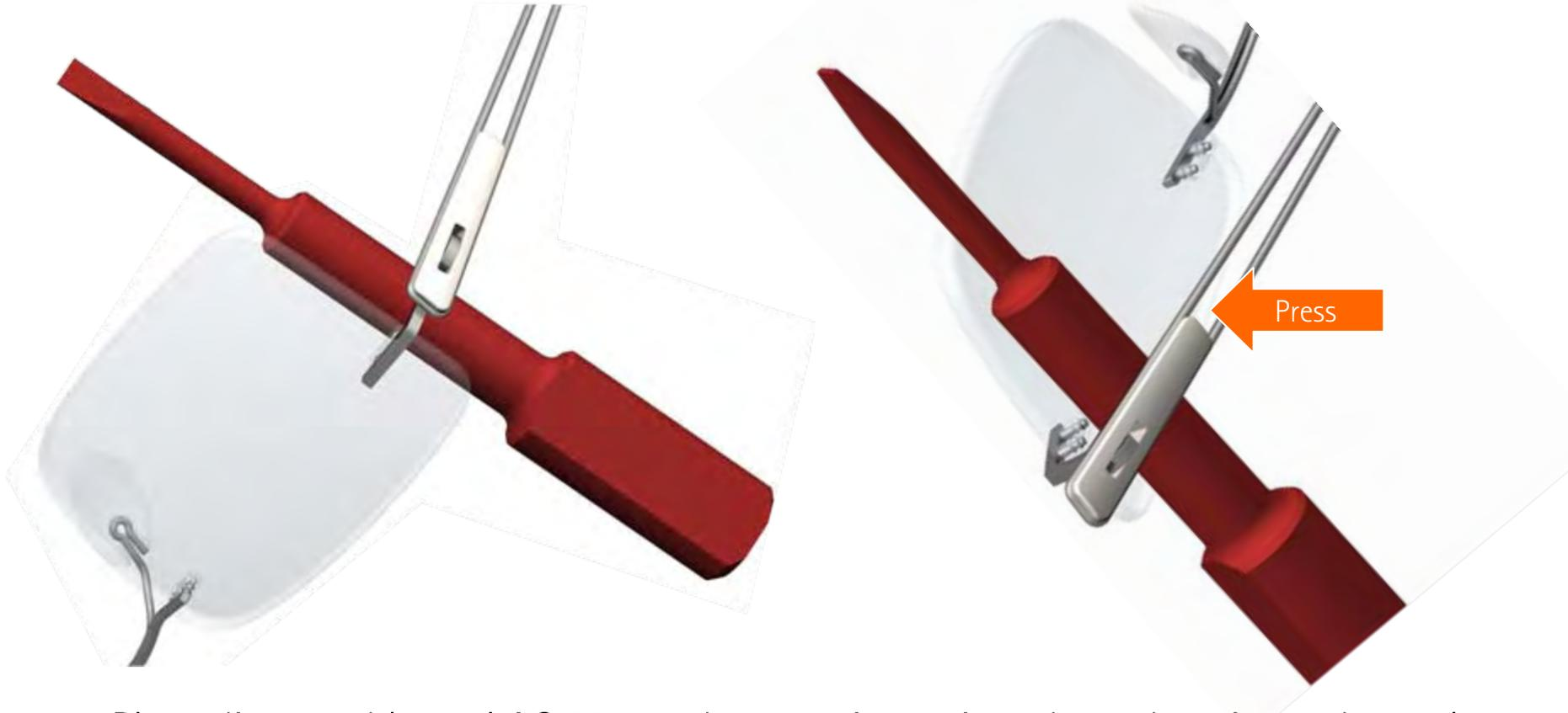
1. Place disassembly tool AC 336 to the stopping point where the trim and temple meet. Select necessary diameter, depending on distance between temple and lens. Close temple and press it through behind the rounded part.
