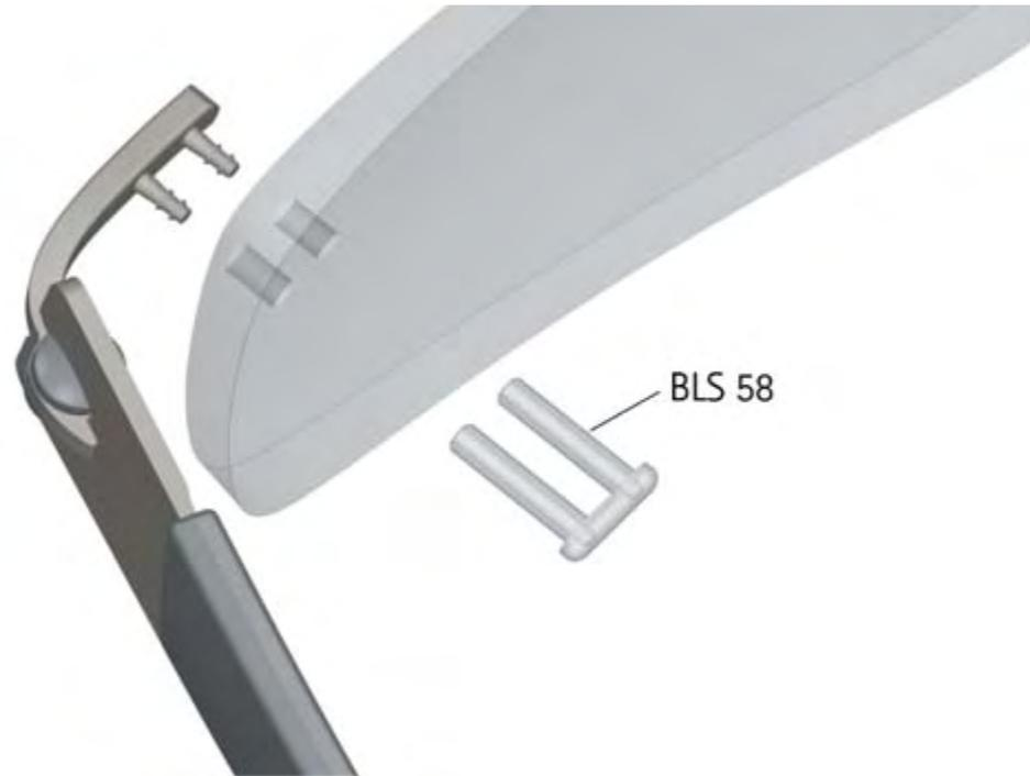
We recommend to glaze principally all metal frames with the harder plastic sleeves BLS 58, especially all models with stiffer temples. Due to the material characteristics and the different construction these sleeves can absorb considerably more tension. This means that the lens fixation holds multiplicatively better.
