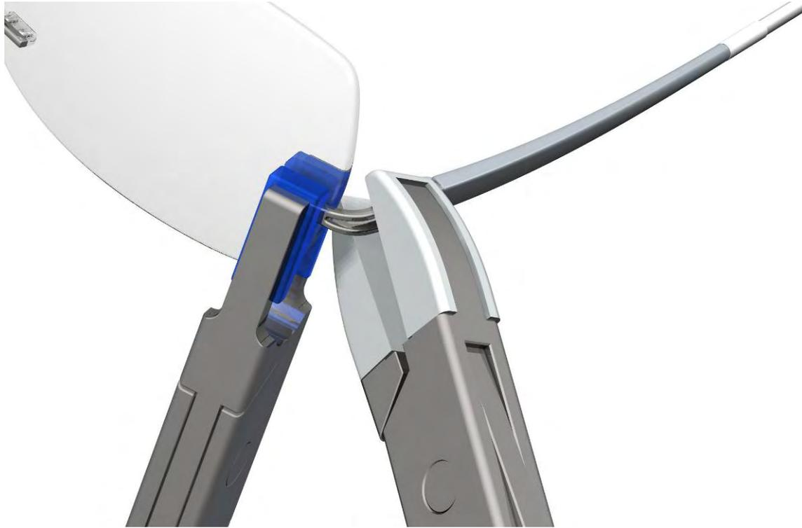
Hold sideparts **very firmly** in the area of the lens fixation with the universal mounting pliers. Incline sideparts with flat pliers.
