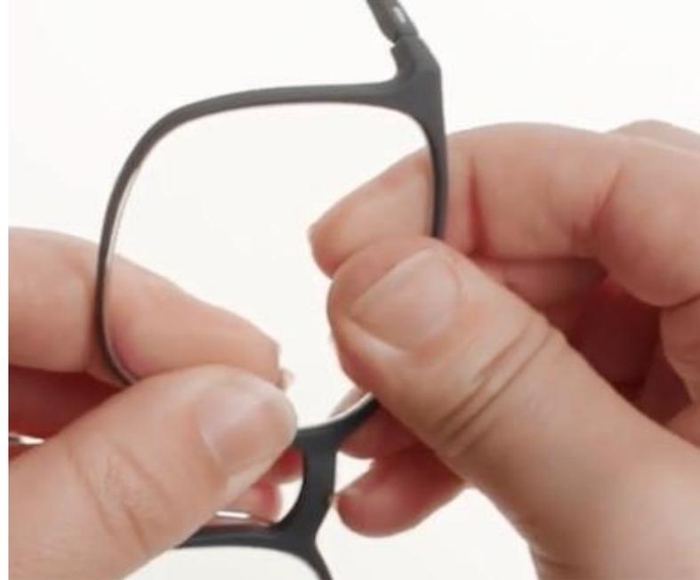
Continue inserting the lens along the top to the nasal side
