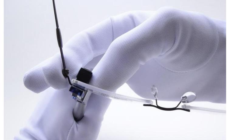
Hold the BLS temple fixation with the mounting pliers and press the temple outward with your thumb or inward with your index finger
