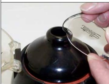
Heat the frame in a limited area only. Holding the lens at the sleeves and the frame at the hinge area.
