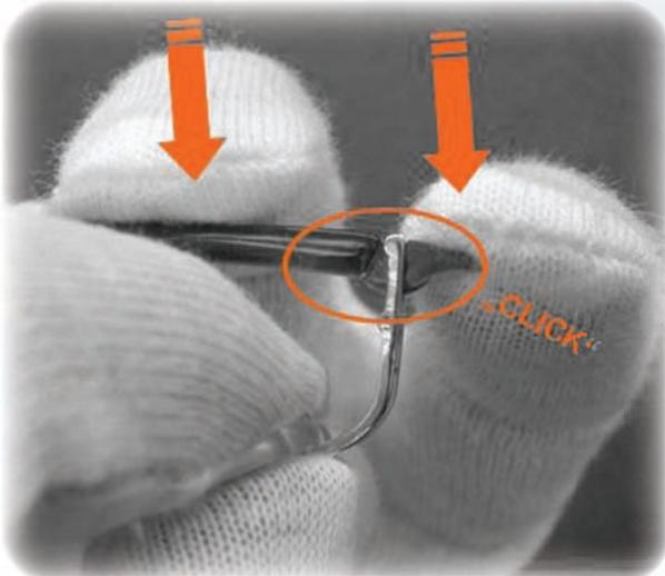
With the temple closed, grip the eyewear firmly at the BLS with thumb and index finger. Press down on the temple on either side of the hinge, and the temple will become unfastened with a click. Remove the temple.
