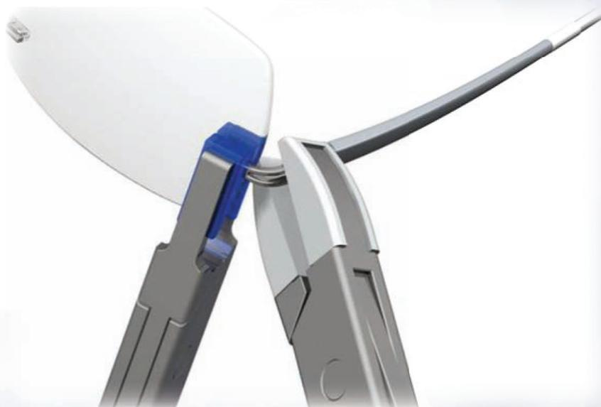
Hold side parts very firmly with the universal mounting pliers close to the area of the lens fixation. Inclinate the side parts with flat pliers. NOTE: Only bend metal parts, never plastic.
