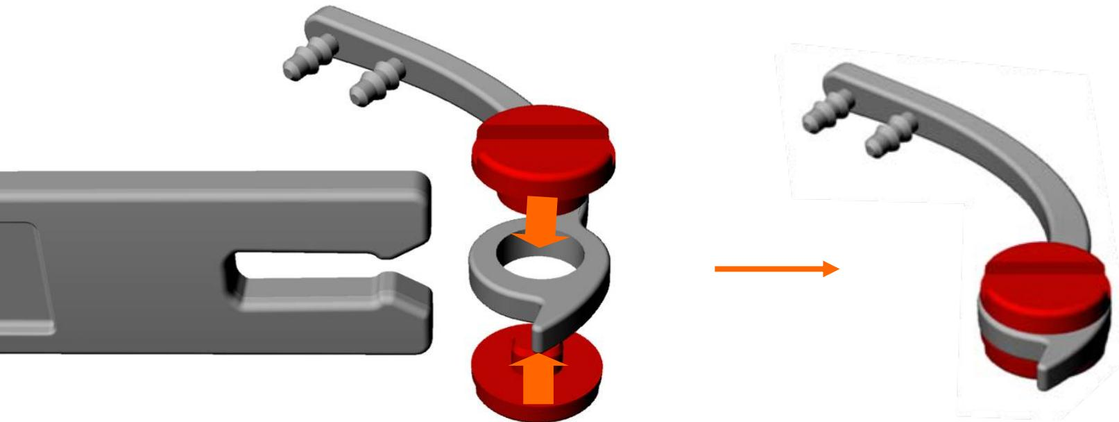
Insert oval hole and oval pivot of plastic hinge on both sides of the loop. The oval shape of the plug-in-system will ensure correct positioning.
