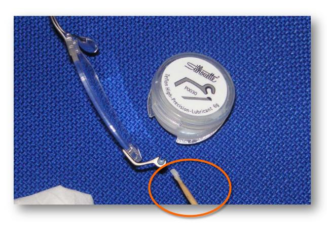
After cleaning, grease inside loop of hinge with high precision lubricant Teflon (P 0030) and mount temple.
