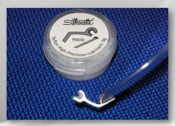
After cleaning, grease inside loop of hinge with Teflon high precision lubricant from mounting box P 0033. Ready to mount temple.
